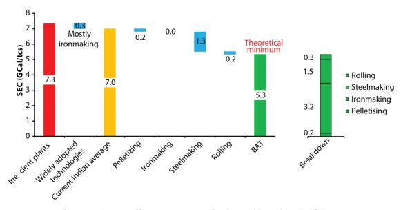
Figure 25: Energy efficiency measures for the coal-based DR-EAF/IF route
